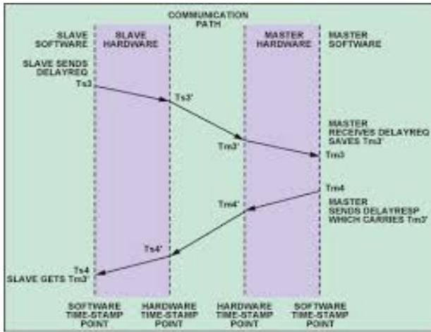
Fig.3 Communication between PTP Master and Slave
