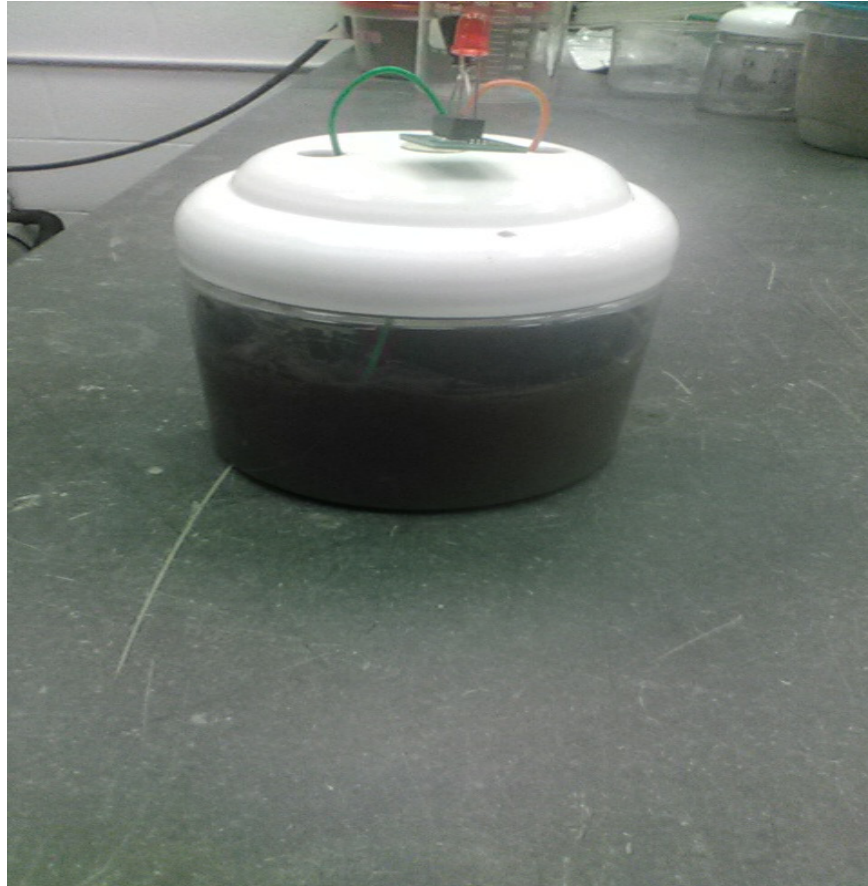
Figure 13. MudWatt MFC container design
