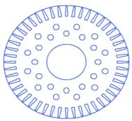
Fig.2 Rotor model of 48 slots developed in RMxprt tool
