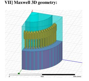
Fig.7 Maxwell 3-D geometry of designed motor
