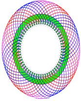
Fig.4 Winding arrangement view in RMxprt tool **III].Performance of Motor:**
