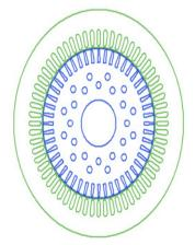
Fig.3 Motor model designed in RMxprt tool
