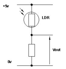
The principle on which these work is that their resistance decreases as the light intensity increases. Typically it is about 1M ohm in darkness, 10K ohm in moderate light and 2K ohm or less in bright sunlight). Because of the relatively high impedance of the analogue inputs on the WASP we can connect the LDR's directly using the circuit shown on the right, where the resistor used is 10K ohm.
