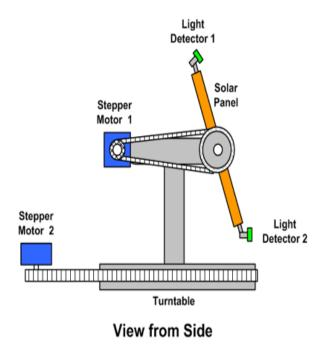
The function of our control system is to move the solar panel in such a way as to keep the received light on each LDR in a pair about the same.
