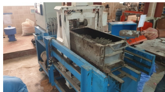
Fig 1 Rolling compactor cum rut analyser
