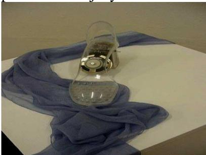
Figure 3.2.2.5 Taser Gun in Shoes Taser guns work the same basic way as ordinary stun guns, except the two charge electrodes aren't permanently joined to the housing. Instead, they're positioned at the ends of long conductive wires, hooked up to the gun's circuit. Pulling the trigger breaks opecompressed gas cartridge inside the gun.
