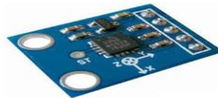
Figure 3.2 Accelerometer
