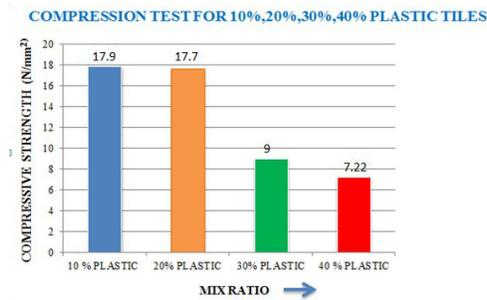
Figure 7 : compressive strength of tile specimens
