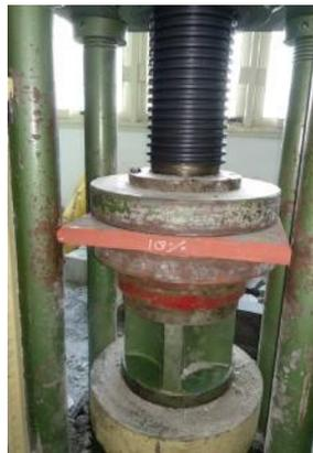
Figure 7 : compressive strength of tile specimens
