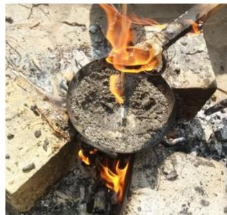
Figure 5 : liquification of plastic in M-sand
