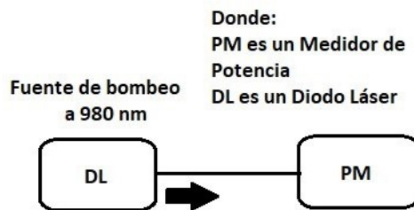
Fig. 1 Experimental arrangement for the characterization of the laser diode.
