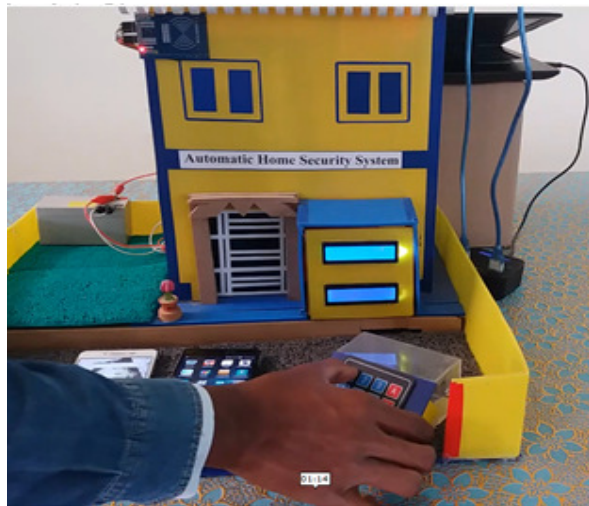
Fig.14 Home Security using Keypad
