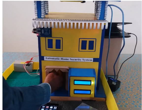
Fig.15 Security Alarm page using Motion Sensor and buzzer
