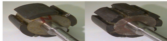
Fig. 4: 4-pole and 8-pole permanent magnet rotor.
