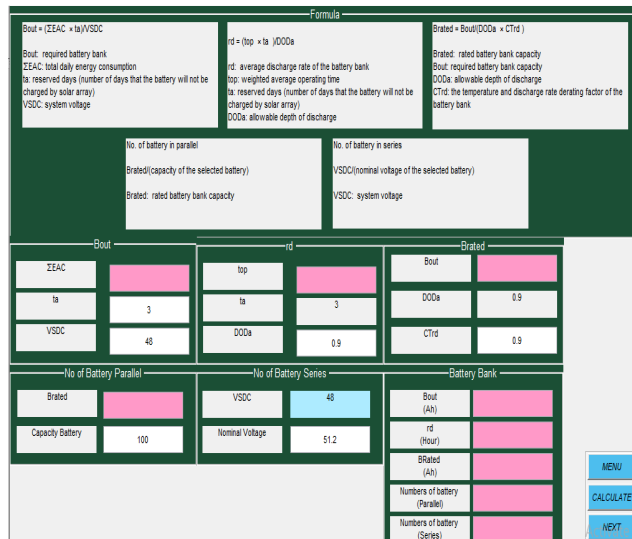
Fig. 7 Battery bank sizing GUI window
