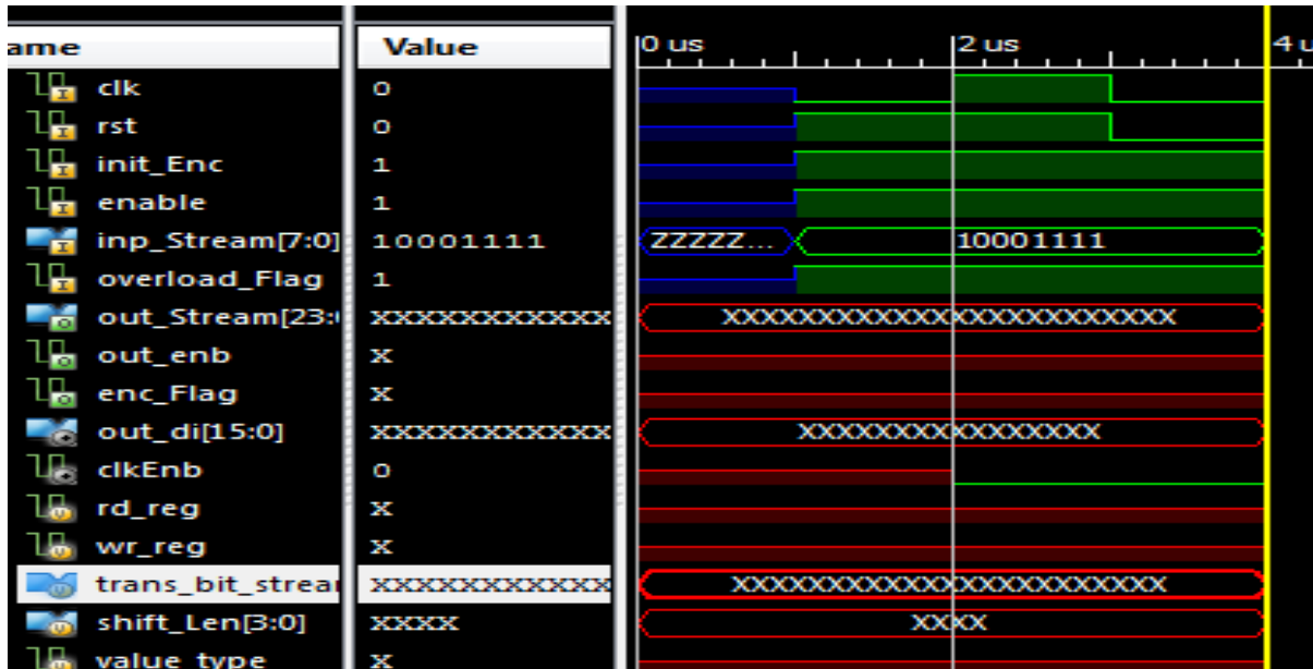
Figure3. Simulation Result of SPIHT Encoder
