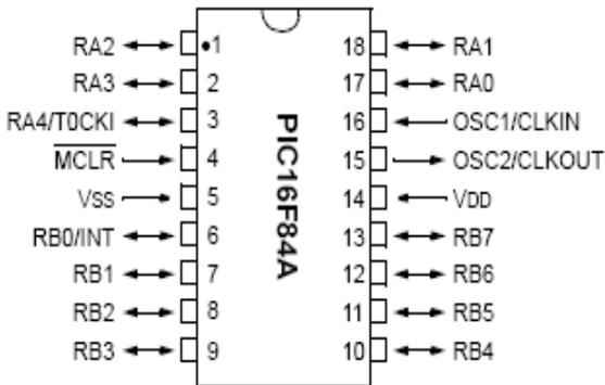
The PIC16F84A belongs to the mid-range family of the PIC microcontroller devices. The program memory contains 1K words, which translates to 1024 instructions, since each 14-bit program memory word is the same width as each device instruction. The data memory (RAM) contains 68 bytes. Data EEPROM is 64 bytes. There are also 13 I/O pins that are user-configured on a pin-to-pin basis. Some pins are multiplexed with other device functions. These functions include:
