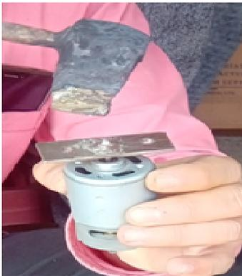
Fig. 7 Mounting of Cutting Blade
