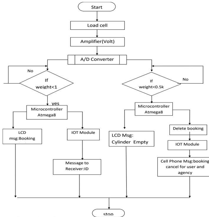
**Flow Chart Gas leakage detection diagram**
