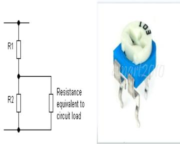
Fig3. Variable Resistor
