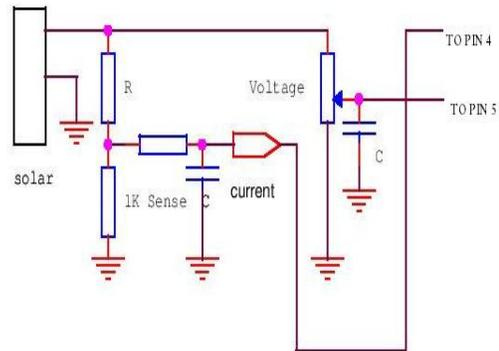
Fig5. overall DC monitoring circuit.
