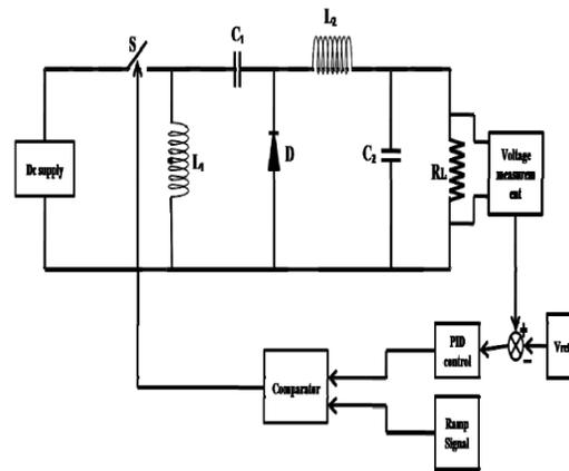
**Fig 4: Open loop simulation of Zeta converter**
