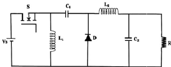
**Fig 1:Proposed structure of Basic Zeta converter**
