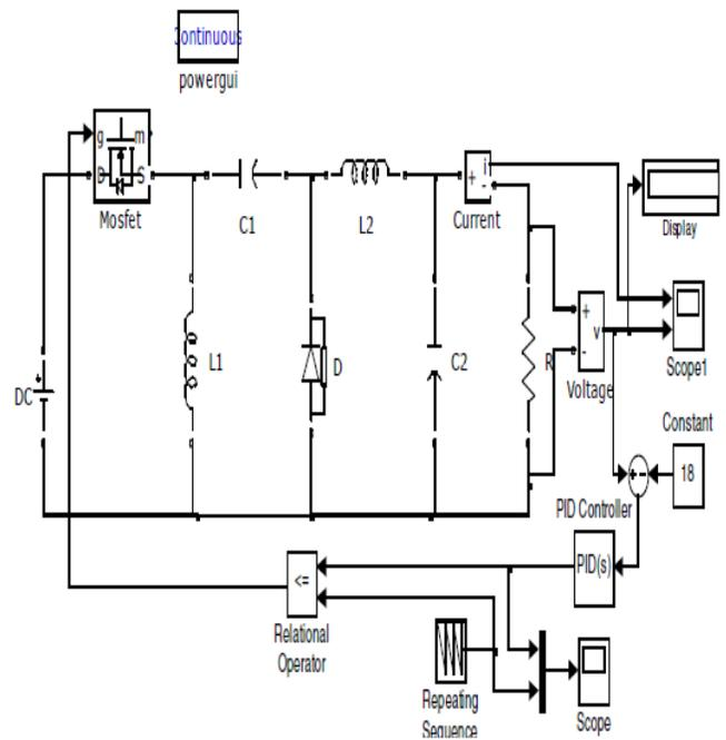
**Fig 5: Closed loop simulation of Zeta converter**
