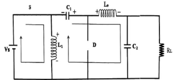
**Fig 2: Zeta converter during MOSFET ON time**
