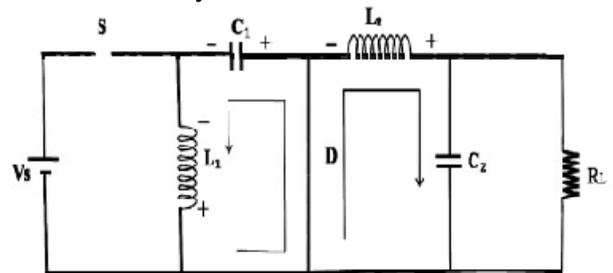
**Fig 3:Zeta converter during MOSFET OFF time**
