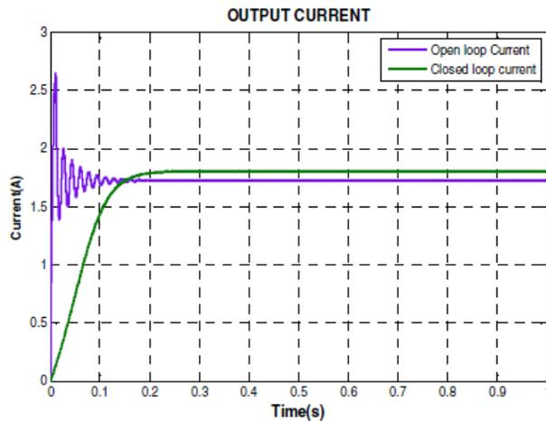
**Fig 6: Output of zeta converter**
