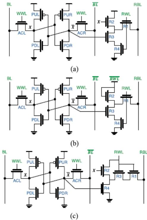
Fig. 2. Schematic of the proposed (a) 10T-P1, (b) 10T-P3, (c) 10T-P2 cells
