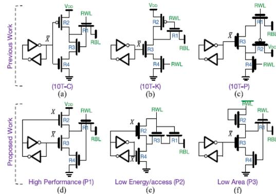
Fig. 3 Schematic of read port of (a) Calhoun and Chandrakasan [1], (b) Kim *et al.* [3], (c) Pasandi and Fakhraie [2], (d) Proposed 10T-P1, (e) 10T-P2, (f) 10T-P3 cell.
