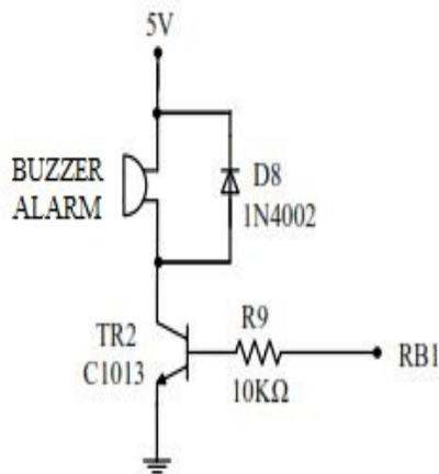
Fig. 4 Buzzer Alarm Circuit
