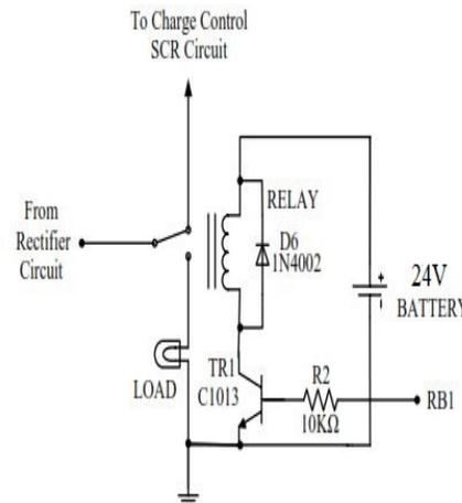
Fig. 3 Relay Circuit for Load Diversion
