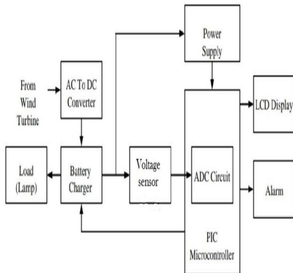
Fig. 1 The Block Diagram of the Charge Controller
