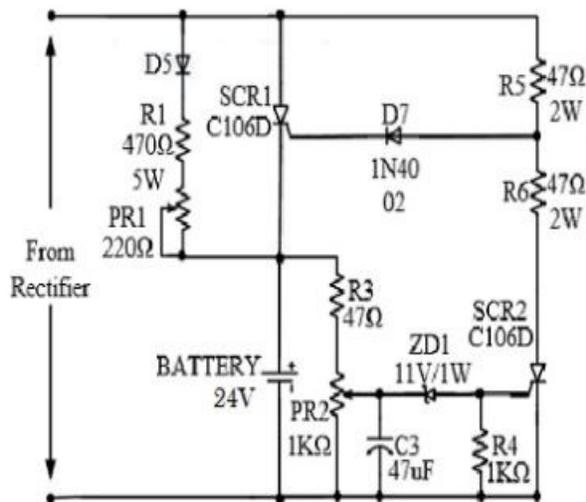
Fig. 2 The SCR Controlled Battery Charger Circuit
