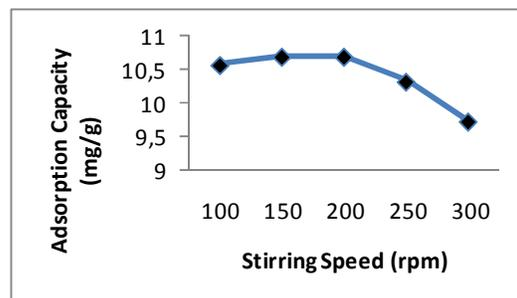
Fig. 4 Effect of stirring speed on absorption capacity of rhodamine B using langsat shell
