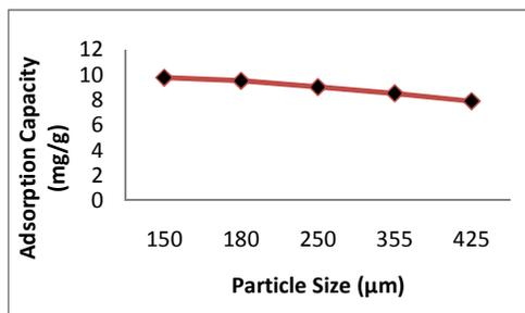
Fig.. 2 Effect of particle size on absorption capacity of rhodamine B using langsat shell
