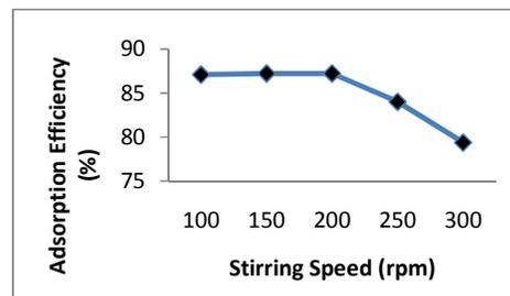
Fig. 5 Effect of stirring speed on adsorption efficiency of rhodamine B using langsat shell
