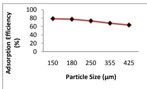
Fig.. 3 Effect of particle size on absorption efficiency of rhodamine B using langsat shell
