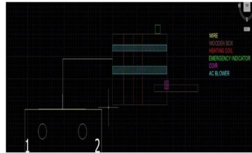
same motor wire, in which the motor and heating coil is operated by a same switch named switch1.
