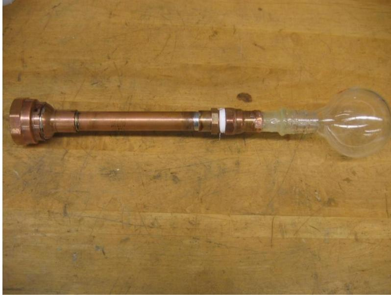
**Figure** Resonator tube with buffer volume
