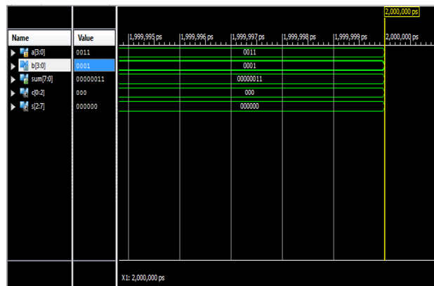
Figure (5): Simulation results of 4-bit multiplier using Pyramidal adder
