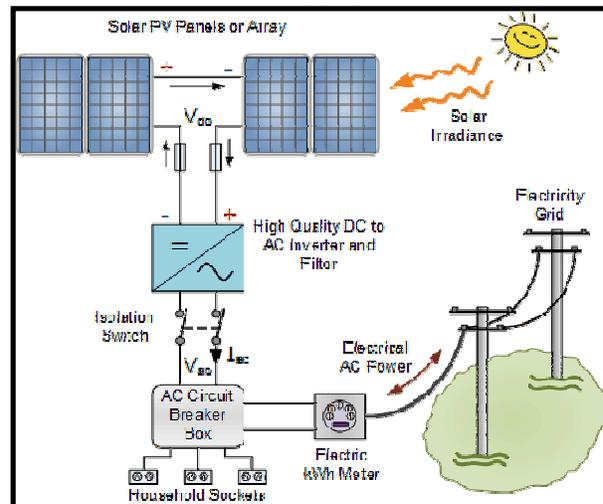
Fig.2 Grid Connected Solar System
