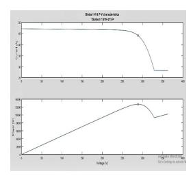
In this case, six strings are connected in parallel and ten modules are connected in series per string. The maximum output voltage and current is 290V & 44.1A respectively. The maximum power output is 12789W.
