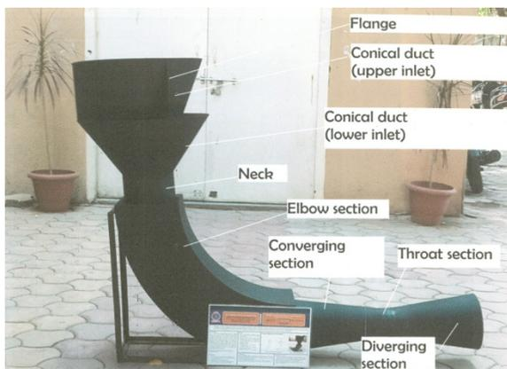
Fig.2 Manufactured DWT Model
