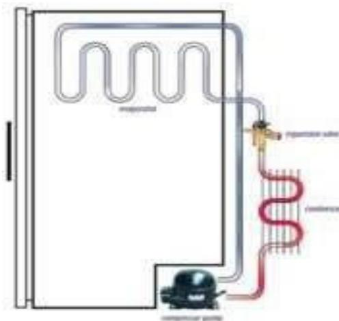
**Fig. 2 Schematic Representation of Refrigerant Flow**
