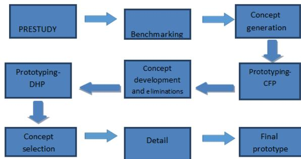
Fig. 1 Schematic diagram of the Product Development Process
