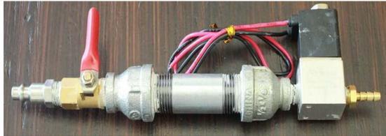
Fig 3. Fuel chamber design
