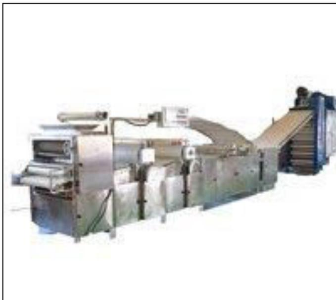
Fig.1 Rolling Automatic Papad making machine
