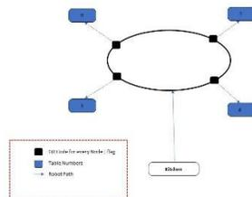
According to the path diagram (shown in figure 3) Navigation Unit (robot) detects the Node using QR Code scanner. The robot navigation unit detect the right node in the path that they travelled, so according to the algorithm robot run on the path circuit and delivered the ordered on each table there will be a QR code could be scanned which will redirect will be directly sent to the kitchen unit.
