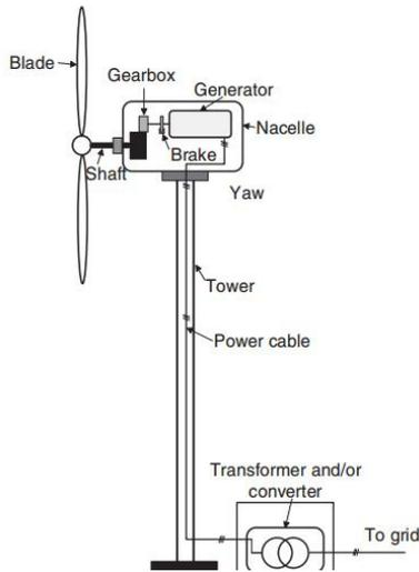
Fig. 1 Structure of a wind power system
