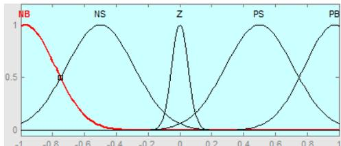
Fig. 10 Membership function of duty cycle
