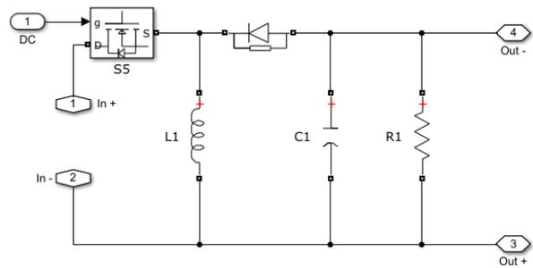
Fig. 2 Buck-Boost Converter Circuit on Simulink
