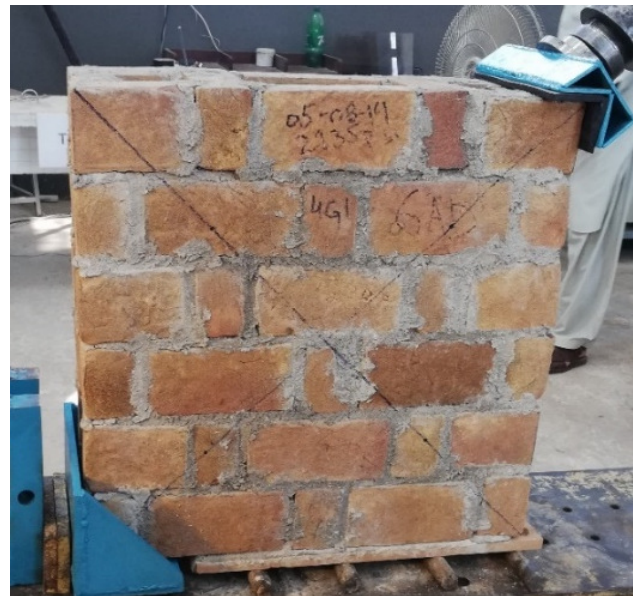
Figure 6 Testing arrangements for diagonal shear strength test
