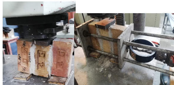
Figure 5 testing arrangements of triplet prisms
