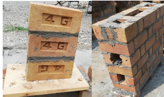
Figure 4 RTB testing specimens triplets and diagonal prisms
