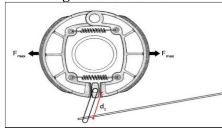
**Fig 3. Drum Brake**
