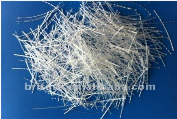
**Figure-1: Polypropylene fiber**
