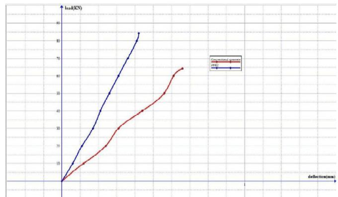
**Figure-5: Test for double shear Deflection vs. Load for M30 Concrete**
