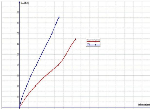
**Figure-6: Test for double shear Deflection vs. Load for M35 Concrete**
