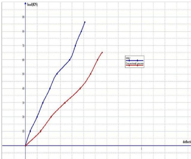
**Figure-7: Test for double shear Deflection vs. Load for M40 Concrete**
