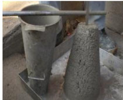
**Figure-1:** Slump Test
