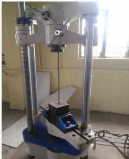
Figure-3: Split Tensile Test
