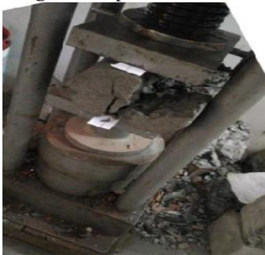
Figure-4: Bond Strength Test
