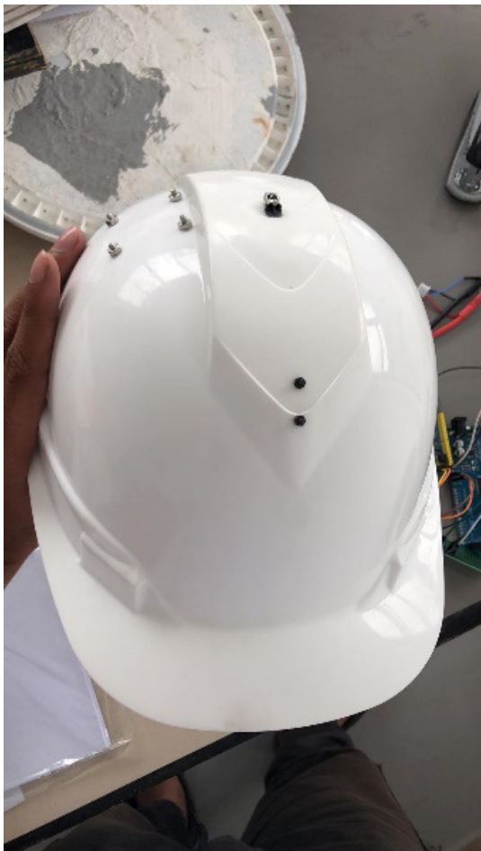
FIG. IIIII HARDHAT WITH INSTALLED SENSORS
