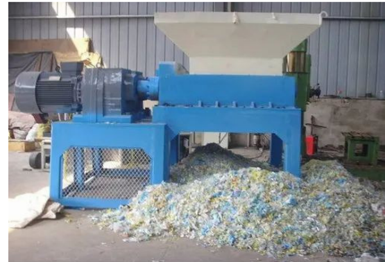
Fig-6: plastic waste by using shredding machine
