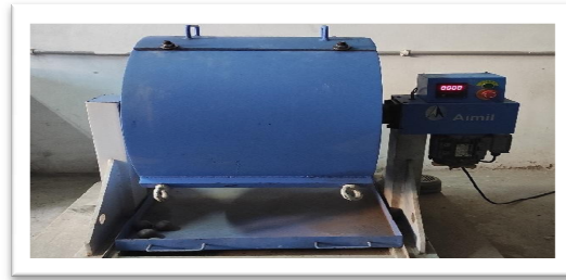
Fig.2 Los Angeles abrasion machine
