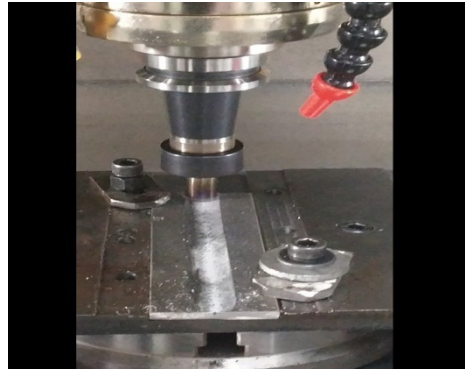
Figure 4.14-4.16 Friction Stir Welding Steps: step1: Plunging step, step2: Stirring step and step3: Retracting step.
