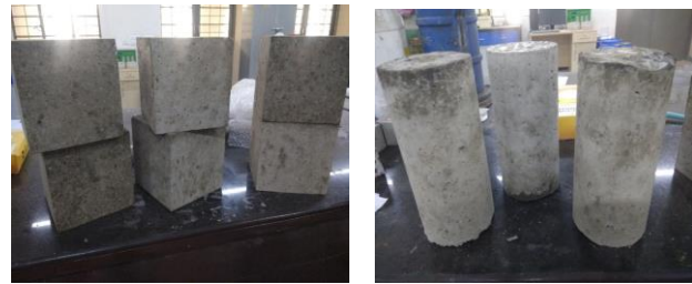
Fig. 11: prepared samples of natural aggregates and RCA
