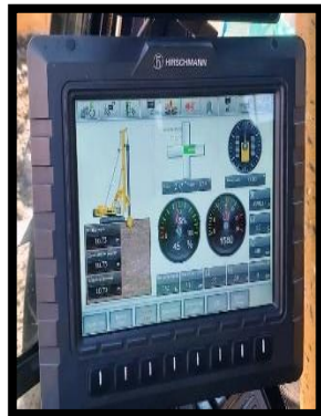
Fig. 3 information screen of Piling Rig Machine
