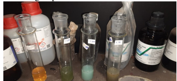
Figure 4.8 After removing the cod digester
