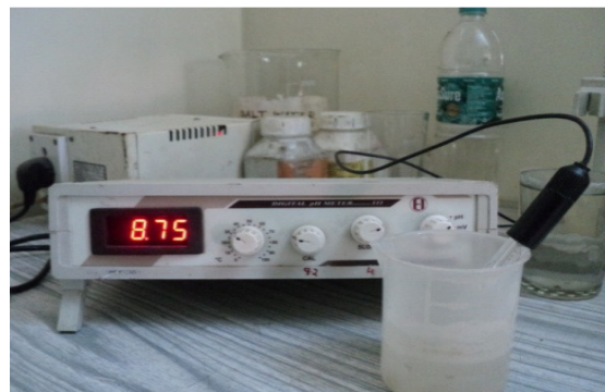
Fig. 8: pH & Potential tests of samples collected
