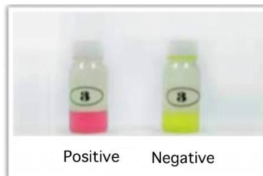
Figure No. 1. The picture showed color metric to interpret result of formaldehyde detection [7]
