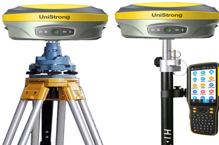
Figure 2.2: UnistrongG970iipro DGPS Used for Field Data Acquisition
