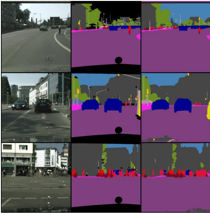
Fig 8: Real image frame (left) vs Ground Truth (middle) vs Predicted Segmentation (right).
