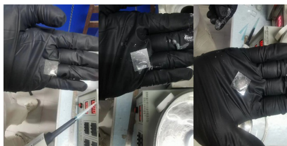
Fig.3 Images of 1-3s spin coating (from left to right )
