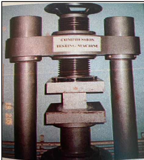
Fig. 1. Compressive Strength Testing
