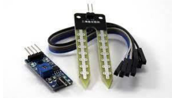
Fig.1 Soil Moisture Sensor
