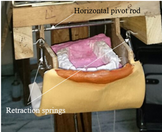
Fig. 33 Jaw of animatronic hardware showing the spring arrangement and pivot rod
