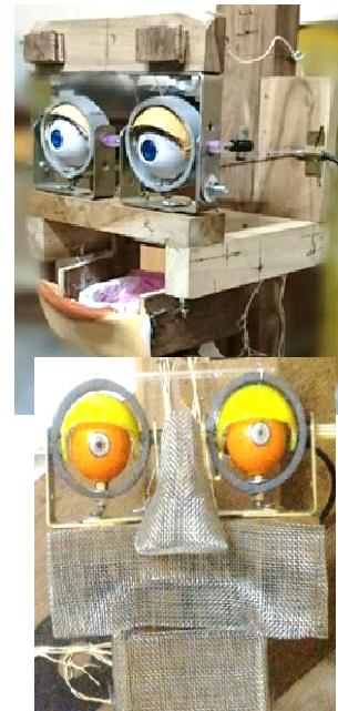
Fig. 36 (Left)Head without mask (Right) shows wire-mesh used to form nose area and upper lip, the curvature of jaw is also formed by wire mesh
