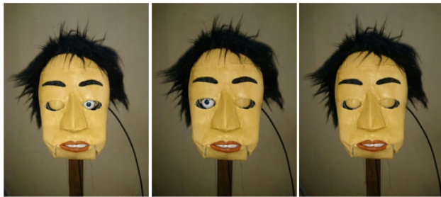
Fig. 40 Model with right, left and both eyelids closed respectively
