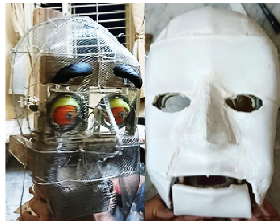
Fig. 37 (Left) shows complete wire mesh mask, the eyebrows are assembled after laying the mask over the frame of head (Right) Foam applied onto the wire mesh and then painted with skin colour to give a human skin look
