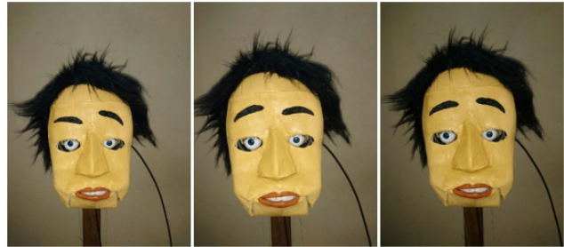
Fig. 42 Model with left, right and both eyebrows raised respectively
