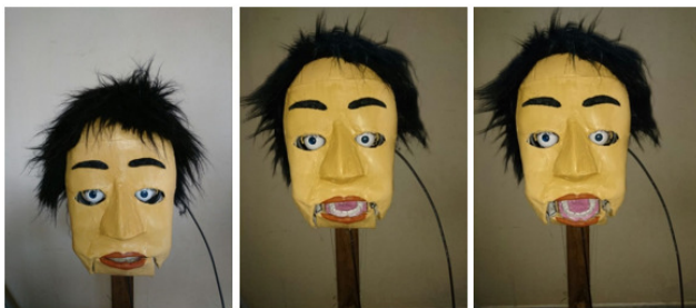
Fig. 41 Model with right, left and both eyelids closed respectively
