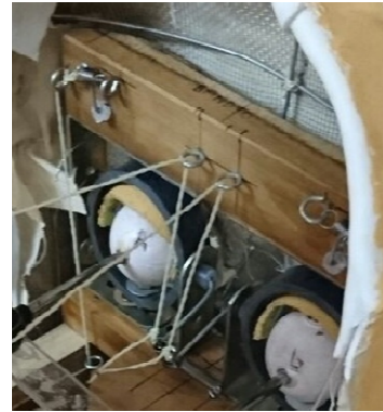
Fig. 34 Crank and spring arrangement for actuating eyebrows
