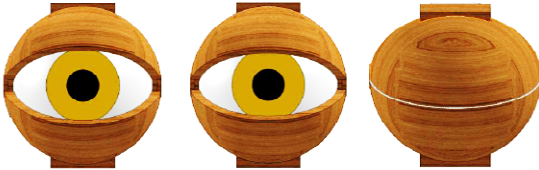
Fig. 16 Various Eyelid Movement, using CAD model
